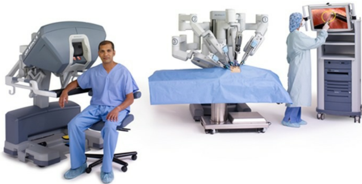
Figure 8 Full da Vinci Si HD Surgical System. From left to right: surgeon console, patient cart, vision cart (31).
